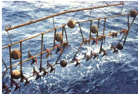
Fig. 1 The plow harrow used during the German large-scale DISCOL-Experiment in 1989 to create a disturbance on the seafloor comparable to a future manganese nodule mining.
