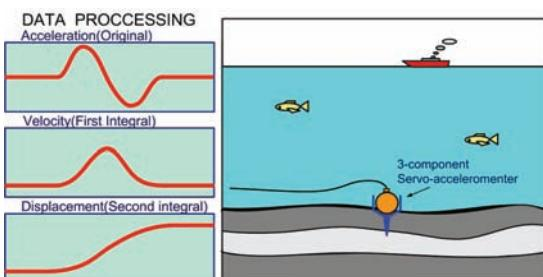
Fig.1 Basic concept of displacement monitoring at the seafloor
