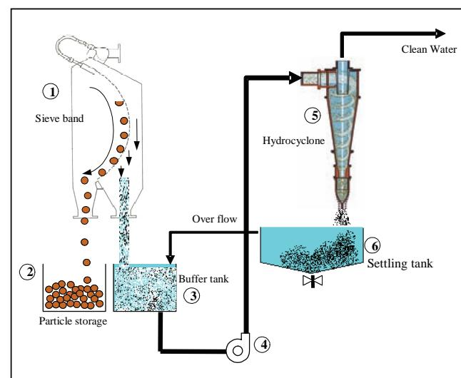
Fig. 1. Schematic diagram of manganese separation using hydrocyclone.
