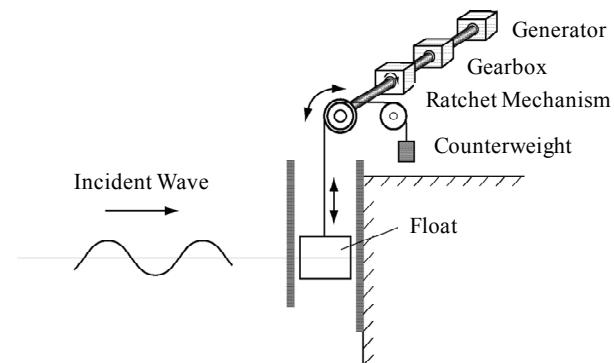
Fig. 1 Schematic diagram of the float-counterweight device
