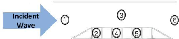
Fig. 3 Diagram showing the structure of the water chambers and the location of wave gauges
