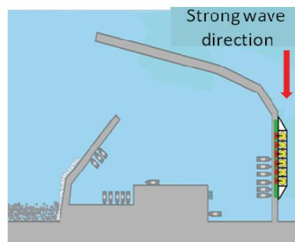
Fig. 2 Conceptual diagram of the location of the water chambers along breakwater
