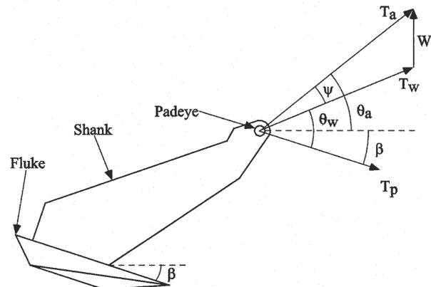
Fig. 1 Anchor force system in clay
