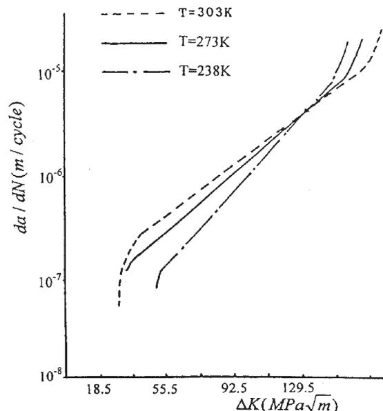
Fig. 1 FCP diagram of steel A537 at different temperatures
