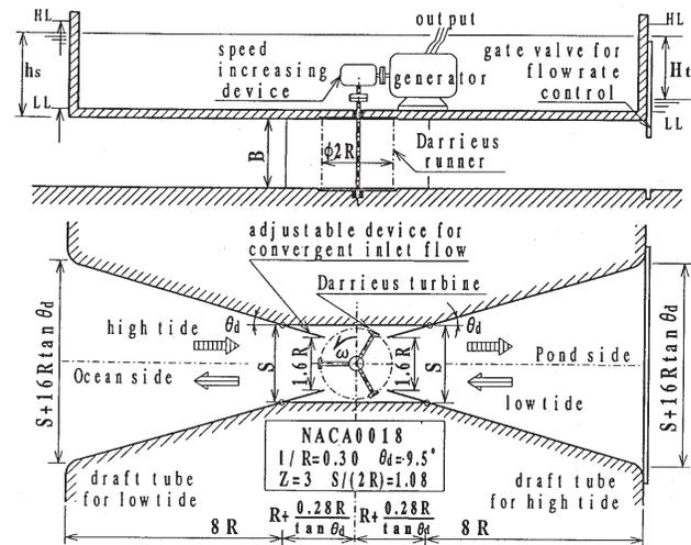
Fig. 1 Schematic view of tidal energy generating system
