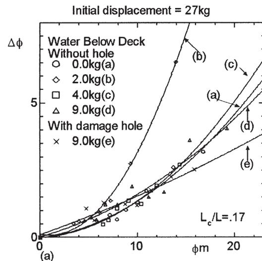
Fig. 1 Roll extinction curve for below-deck flooding
