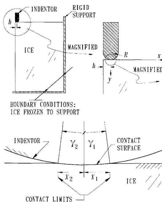
Fig. 1 Initial contact between semicircular indentor and ice
