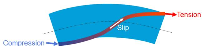
Fig. 1 Slip of helical elements due to bending
