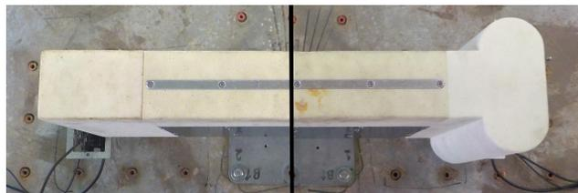
Fig. 2 40th scale model of common box-shaped flap shown without (left) and with (right) end-effectors
