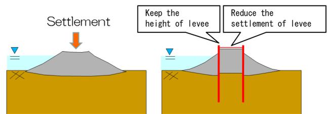
Fig. 1 The effectiveness of the double sheet-piles countermeasure
