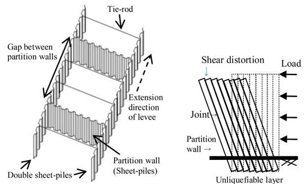
(a) Double sheet piles with partition walls (b) Shear distortion
