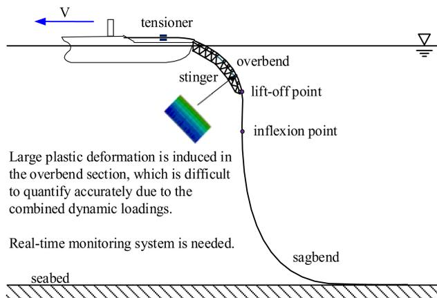
Fig. 1 S-lay operation
