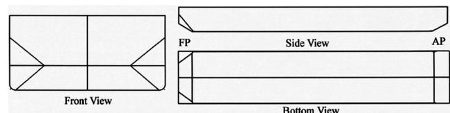
Fig. 1 A box-shaped FPSO hull
