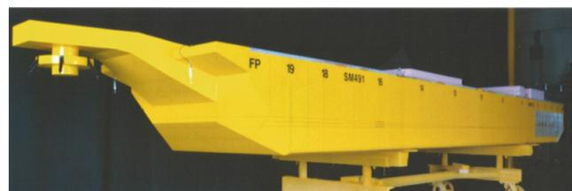
Fig. 2 FPSO model (1/60 scale)
