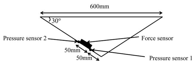
Fig. 1 Section of the wedge
