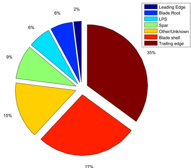
Fig. 1 Blade defects
