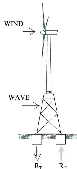
Fig. 1 A wind turbine on a jacket with several bucket foundations with reactions to tensile loading ( $R_T$ ) and compressive loading ( $R_C$ )
