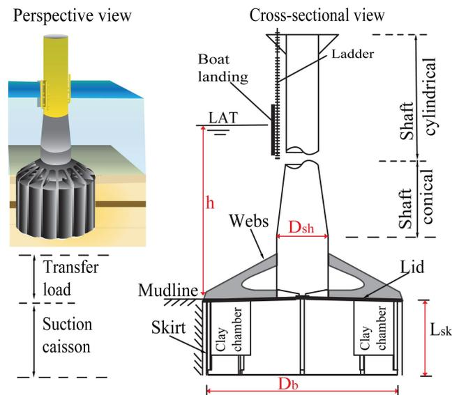
Fig. 1 Perspective and vertical cross-sectional view of Mono Bucket foundation
