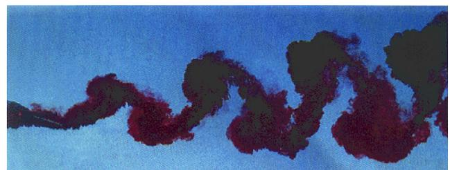
Fig. 1 Jet flow and reverse Karman street visualized through dye behind a tuna-shaped swimming robot (Triantafyllou and Triantafyllou, 1995)
