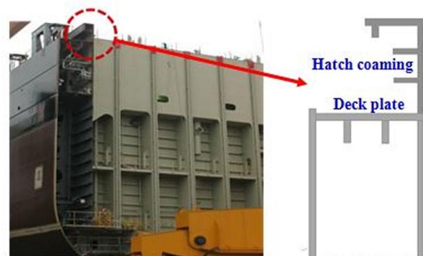
Fig. 1 The upper structure of a large container ship and applied steel plates
