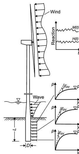
Fig. 1 Schematic sketch of an OWEC with a monopile foundation
