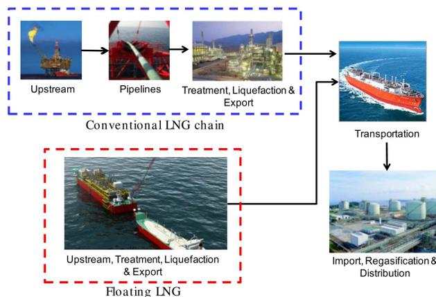
Fig. 1 Concept of Floating LNG and LNG supply chain (Song, 2012)
