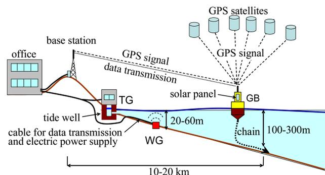
Fig. 1 NOWPHAS equipment for tsunami observation
