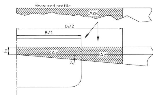
Fig. 1 Measured brash ice channel (from FSICR, 2005)
