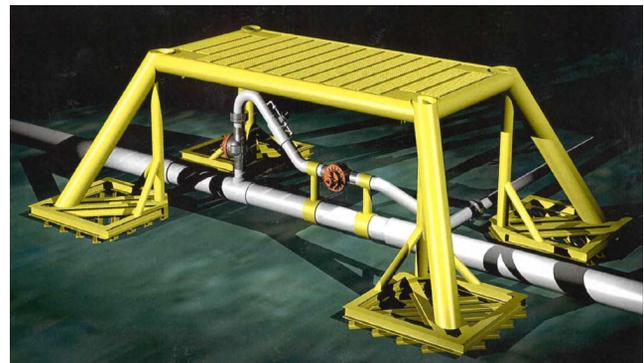
Fig. 1 Typical subsea hot-tap connection
