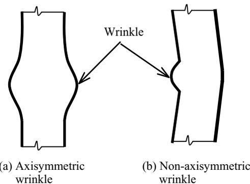
Fig. 1 Typical bulge wrinkle shapes
