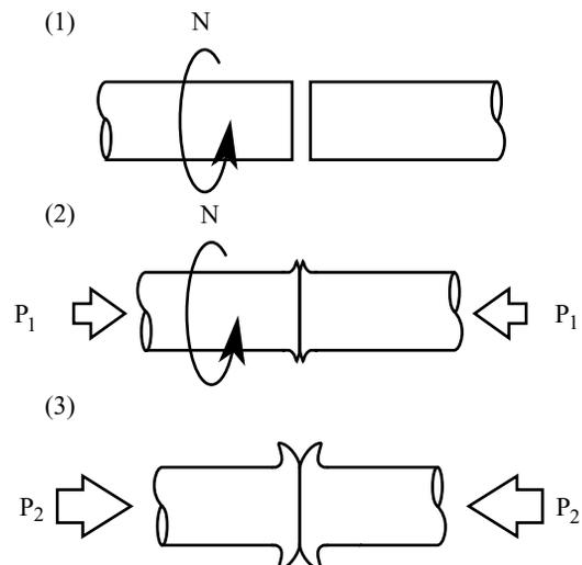
Fig. 1 Basic steps in friction welding process
