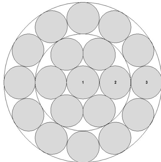
Fig. 2 Self-damped cable cross-section
