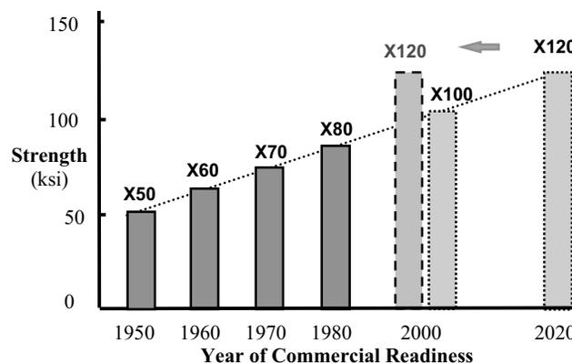
Fig. 1 Evolution of linepipe technology (ksi/0.145 = MPa)
