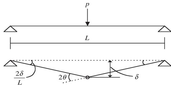
Fig. 1 Plastic collapse of simply supported beam
