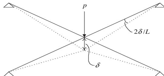
Fig. 2 Plastic collapse of 1 x 1 grid
