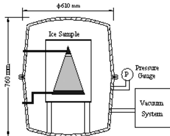
Fig. 1 Schematic diagram of evacuated chamber
