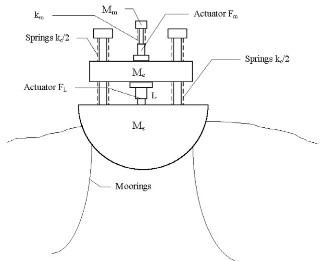
Fig. 1 Schematic of compensator system in heave
