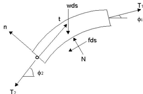
Fig. 1 Mooring line and free body diagram
