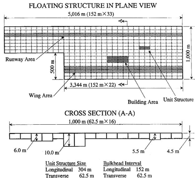
Fig. 1 Floating structure, Mega-Float
