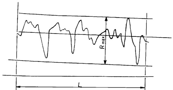
Fig. 1a Definition of roughness  $R_{max}$  (JIS, 1982)
