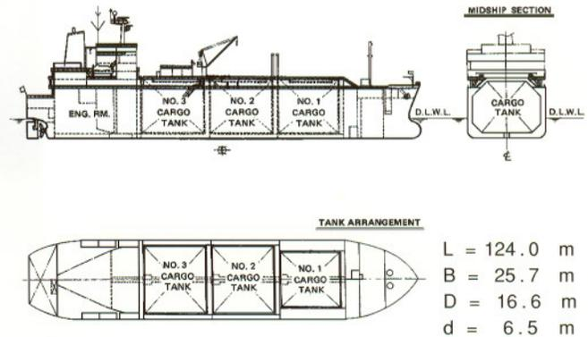
Fig. 1 General arrangement of 18,800 M<sup>3</sup> LNG carrier
