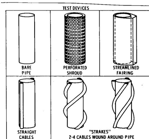
Fig. 1 Three basic configurations of vortex-suppression devices
