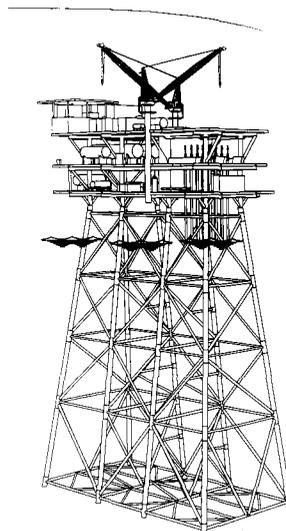
Fig. 1 Typical fixed offshore platform
