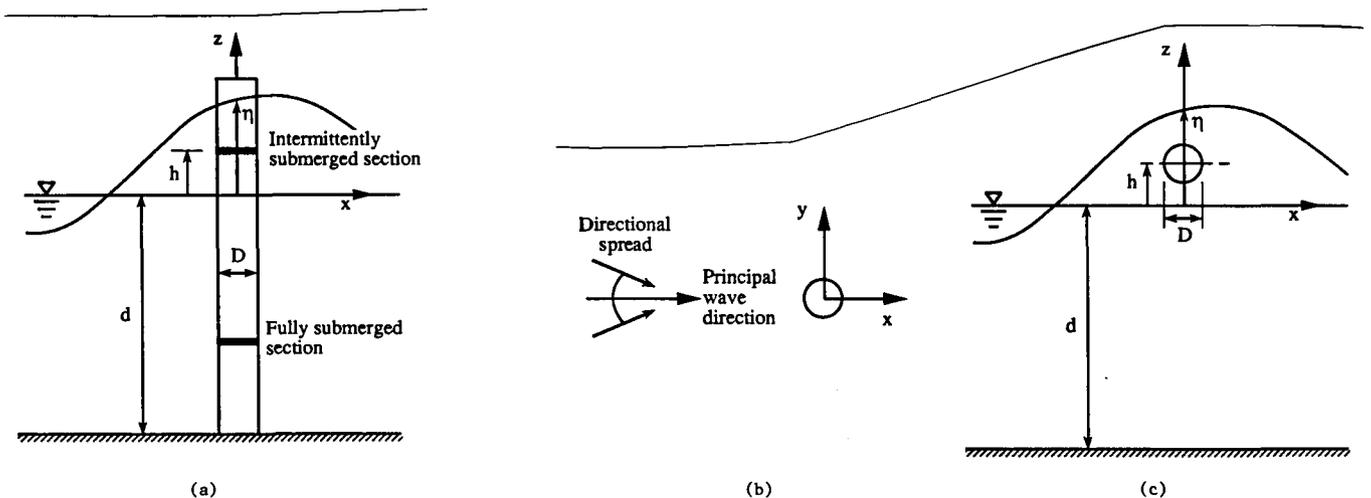
Fig. 1 Definition sketches. (a) random waves past fully and intermittently submerged sections of a vertical cylinder; (b) multidirectional random waves past a vertical cylinder; (c) random waves past a horizontal cylinder near the free surface.
