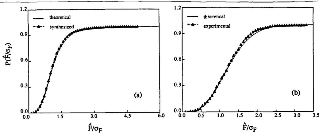
Fig. 3 Comparison of theoretical, synthesized and experimental probability distributions of force maxima for short-crested waves ( $s = 1$ ). (a) theoretical and synthesized distributions; (b) theoretical and experimental distributions.
