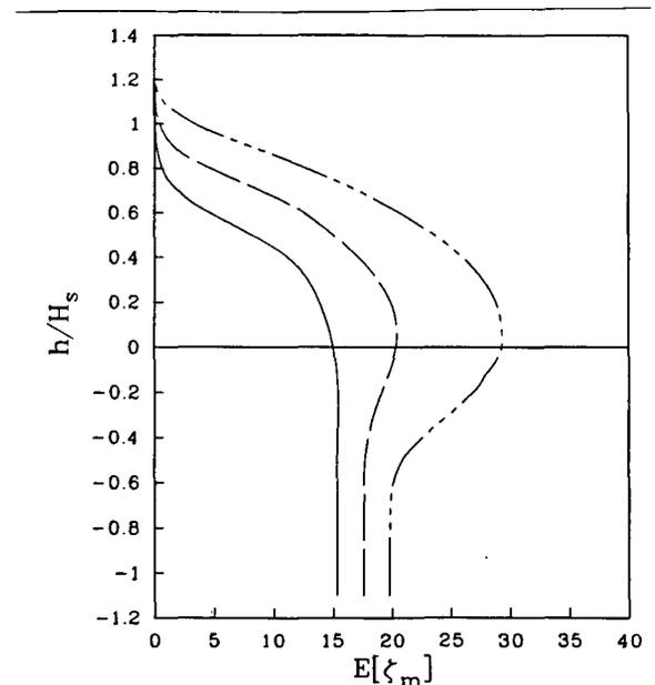
Fig. 6 Vertical distributions near the still water level of the expected value of the largest maximum  $E[\zeta_m]$  of the vertical force on a horizontal cylinder for a duration of  $N$  waves. —,  $N = 10$ ; ---,  $N = 100$ ; - · - · -,  $N = 1000$ .
