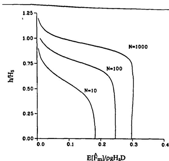
Fig. 4 Vertical distributions above the still water level of the expected value of the largest maximum of the sectional force on a vertical cylinder for a duration of  $N$  waves.
