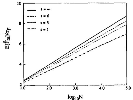
Fig. 2 Expected values of the largest force maximum as a function of  $N$  for long-crested and short-crested waves.
