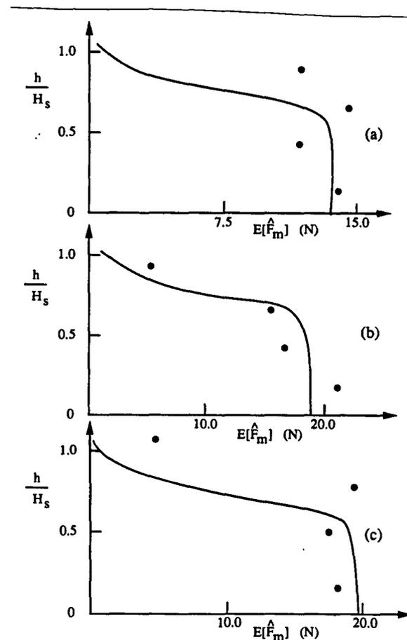
Fig. 5 Comparison of measured and predicted vertical distribution of the largest force maximum above the still water level for three wave conditions. (a)  $T_p = 3.13$  s,  $H_s = 0.43$  m; (b)  $T_p = 2.44$  s,  $H_s = 0.39$  m; (c)  $T_p = 1.96$  s,  $H_s = 0.31$  m. —, theoretical; •, measured.
