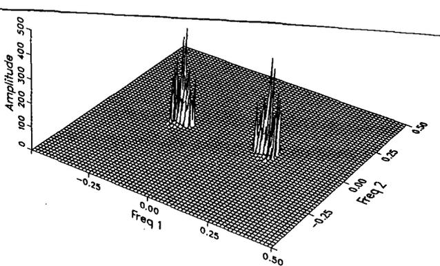
Fig. 4 Surge force quadratic transfer function ( $\text{kN/m}^2$ )
