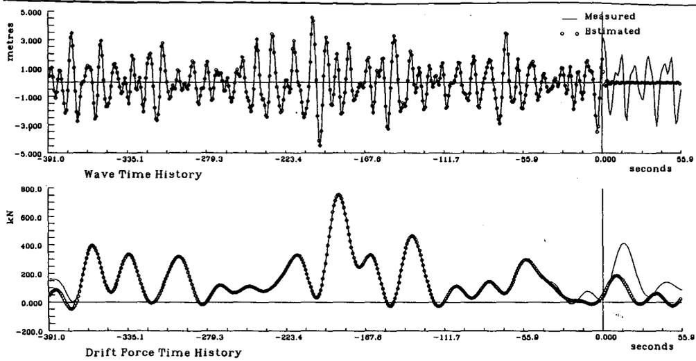
Fig. 6 Real time estimation of simulated wave and drift force
