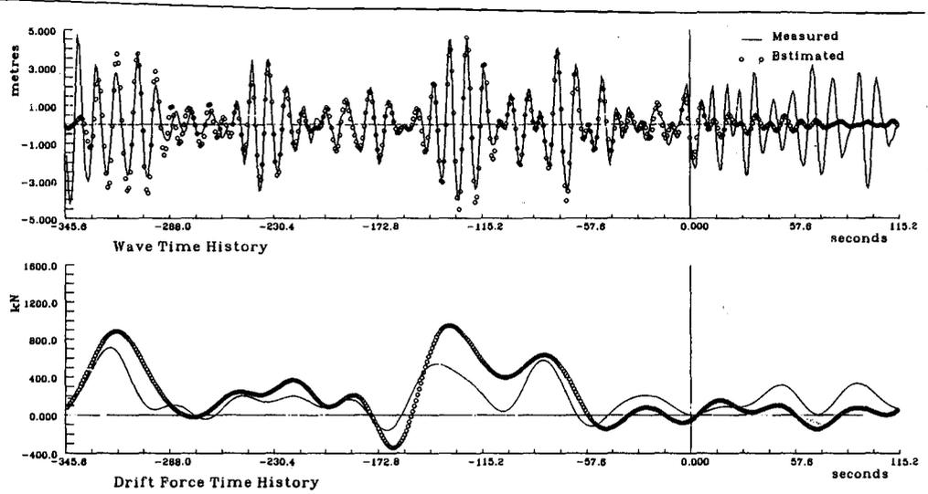
Fig. 5 Real time estimation of experimental wave and drift force
